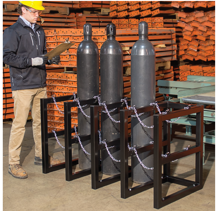
Secure and store cylinders in a barricade rack—visually inspect on a routine basis for any indication of leakage or problems.
